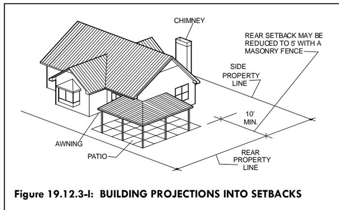
**Figure 19.12.3-I: BUILDING PROJECTIONS INTO SETBACKS**
