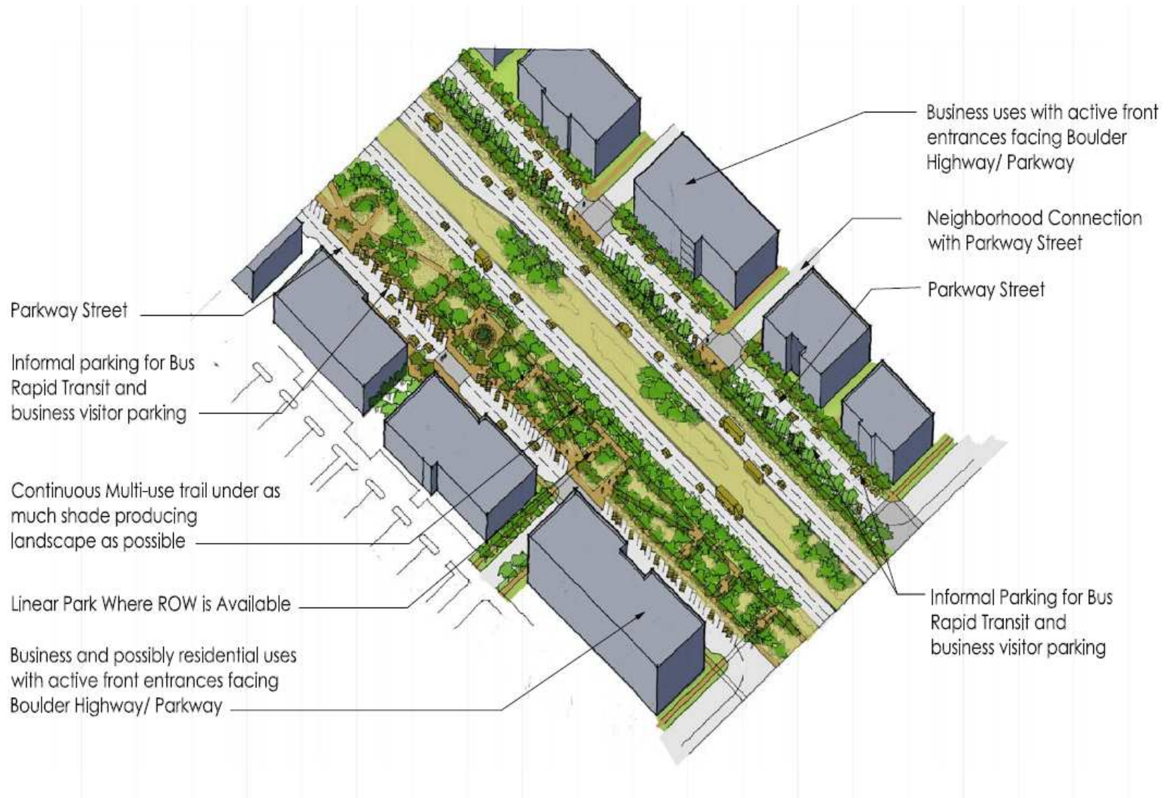
Figure 16—Parkway Street Concept: Axonometric
